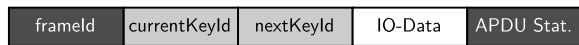
Figure 8. PROFINET IO RTC frame with additional currentKeyId and nextKeyId fields for rekeying purposes.
